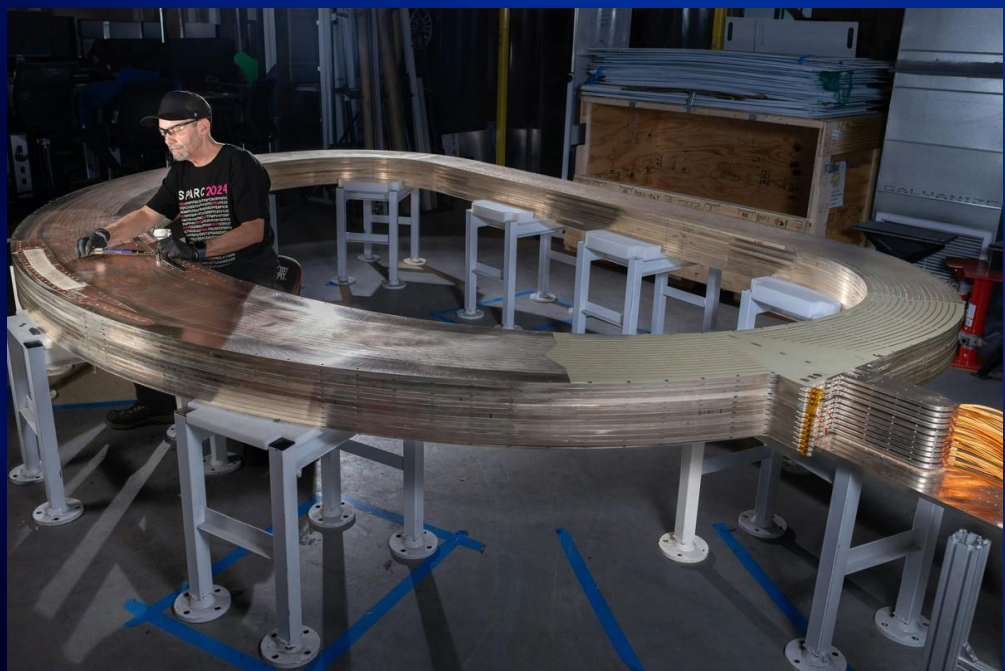
HTS magnet: Commonwealth Fusion Systems (MA)
